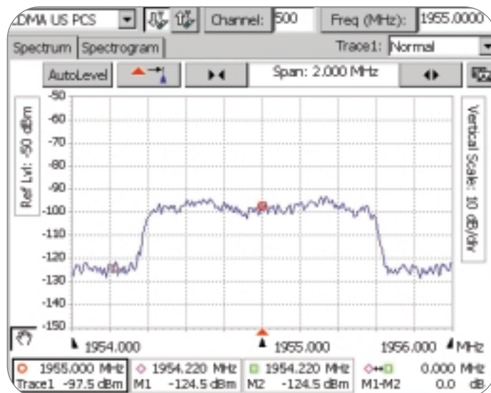
► Figure 23. CDMAOne (using 2 MHz span).
