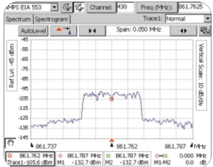
► Figure 26. SMR (specialize mobile radio) signal.
