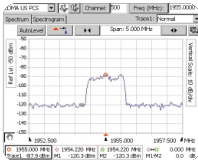
► Figure 22. CDMAOne (using 5 MHz span).
